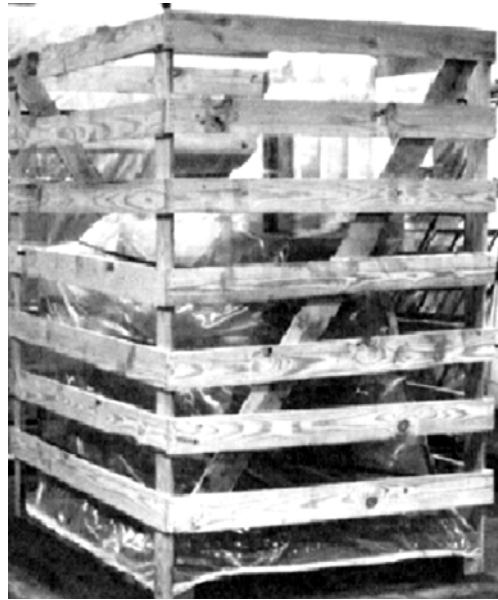
Typical Crating and Cover for a Core and Coil Assembly
