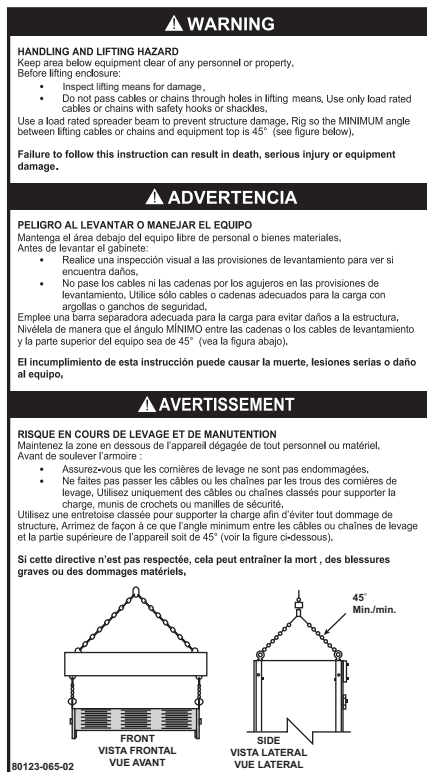
Label Applied Adjacent to Lifting Eyebolts
