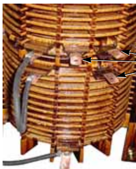
Figure 10: Disk Wound Tap Connections
