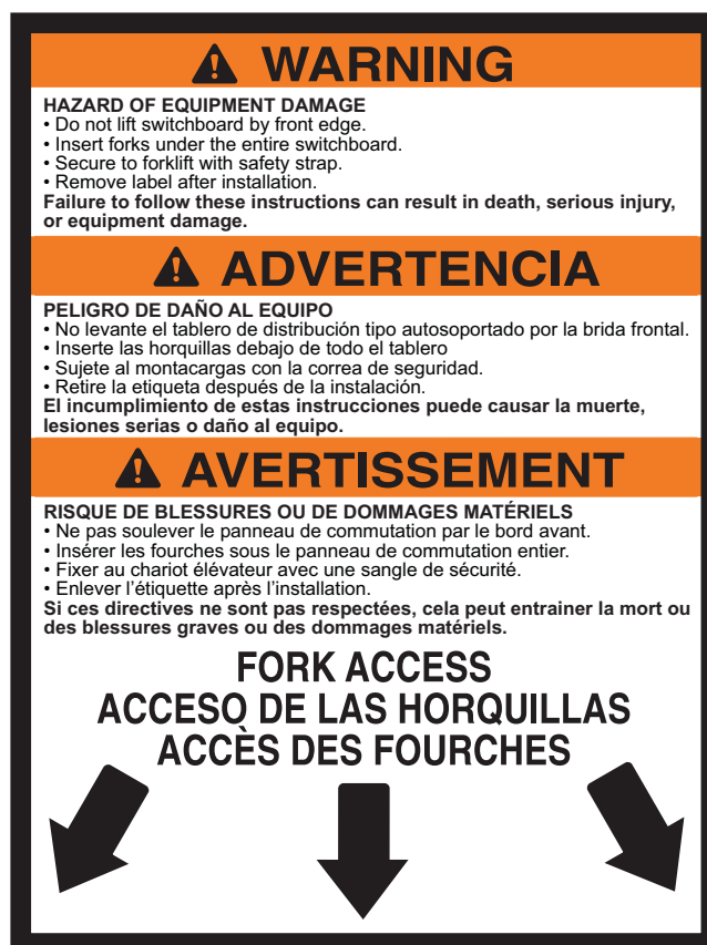
Figure 2 – Warning Label, Rainproof Switchboards
